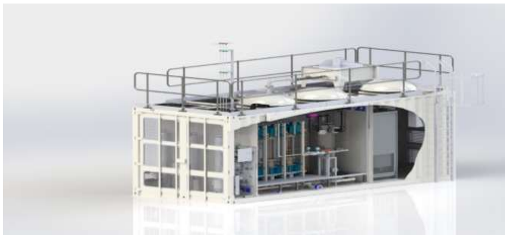
Figure 4 Render of substation of electrolyser
